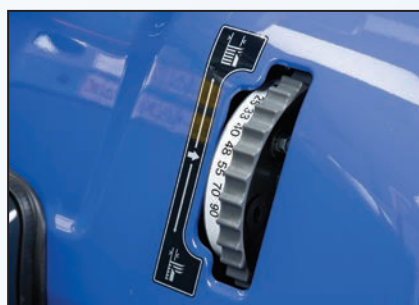
"Dial-in" cutting height adjustment
