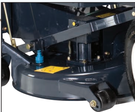
Gear drive to rotary blades and hose-lock fitting for washing/washout
