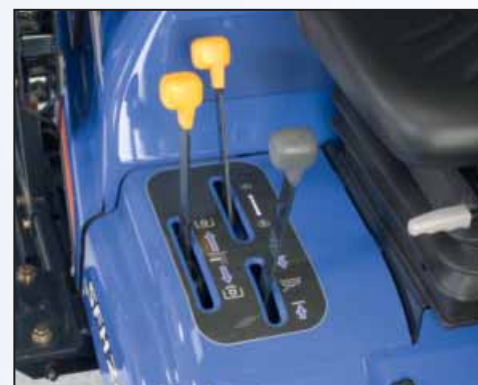
Levers fall readily to hand for deck lift/low, PTO to blades and blower
