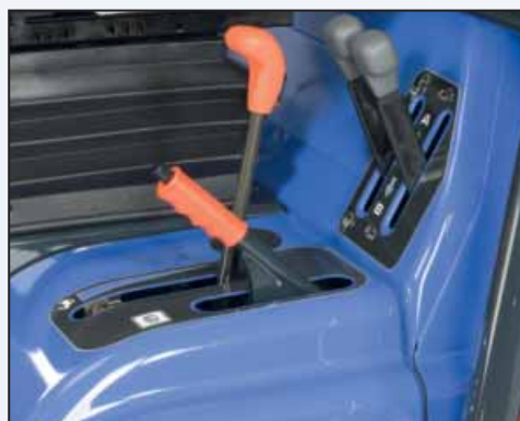
Easy to use parking brake, and levers for emptying the high dump collector
